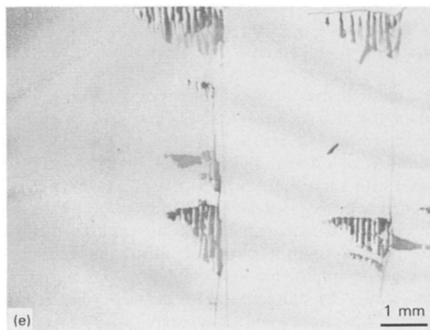
Figure 3 (a) Smooth separation mode (SEM), (b) groove separation mode (SEM), (c) flat silicon breakage (optical microscopy), (d) flat breakage mode (SEM), (e) long fracture mode (optical microscopy).
